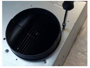
2. Remove the 2 rear screws that hold the motor housing to the back of the
