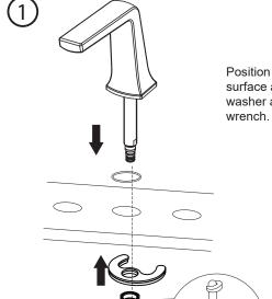
Position the body with o-ring on the installation surface as shown and secure it with metal washer and tighten the lock nut with basin wrench.
