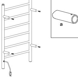
• Insert screw (b) to connecting tube (a).
