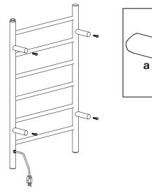
• Insert screw (b) to connecting tube (a).
