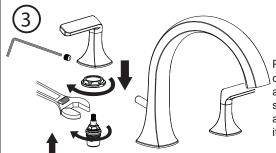
Place a new cartridge in the cartridge seat, then screw the base and assemble the handle by securing the screws. Repeat the above steps for the other cartridge if necessary.
