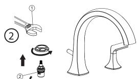
Unscrew the old cartridge② with Adjustable Wrench①, then take it out.
