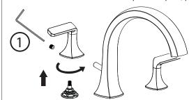
Remove the handle counter clockwise, as shown.
