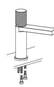
• Place the faucet (3) on the deck and tighten the mounting poles(4)
