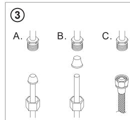
Connect to water supply lines with either: (A) 3/8'' O.D.copper tubing (ball nose risers with the coupling nuts or; (B) 3/8'' copper tubing (no ball) with supplied tube head interior connector or; (C) IPS faucet connectors (1/2'').
