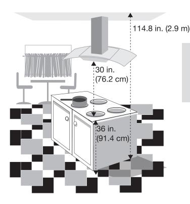
Maximum ceiling clearance 114.8 in. (2.9 m) at 30 in. (76.2 cm) hood mounting height above countertop or stove (May vary with different model). Chimney extensions available for higher ceiling.
