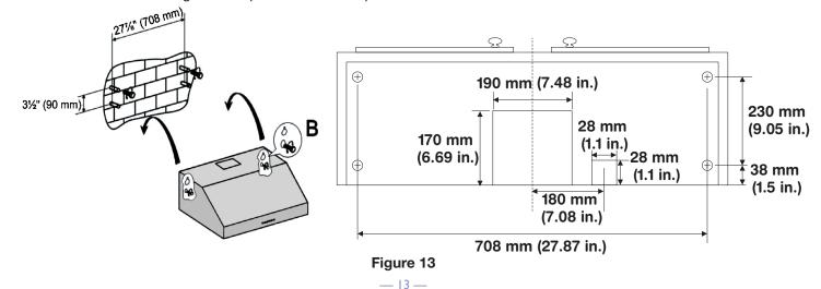
Method 2: attach the ducting to the rear rectangular damper and exhaust outdoors.
