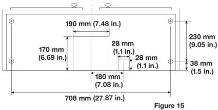
**Method 4:** attach the range hood under the kitchen cabinets and ducting to the rear rectangular damper and exhaust outdoors.
