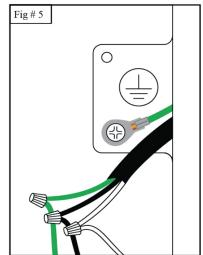
SAFETY WARNING: Risk of electrical shock. This range hood must be properly grounded. Make sure this is done by a qualified electrician in accordance with all applicable national and local electrical codes. Before connecting wires, switch power off at service panel and lock service panel to prevent power from being switched on accidentally.
