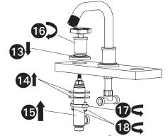
•Place the base on the deck (13) and put on the mounting gasket and iron (14).
