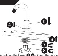
•While holding the base (3,4), insert the faucet body in the deck (5) and reattach the mounting gasket and iron under the deck with the nut removed in step 1.
