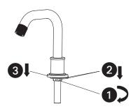
•Remove the nut (1) that holds the mounting gasket in place and remove the mounting gasket and iron (2).
